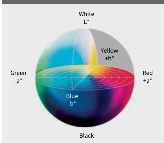
FIGURE 3. CIE 1976 L^*a^*b^* idealised uniform colour space
